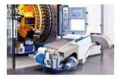
Moveable and adjustable (in height and angle) infeed and exit conveyors for good access
