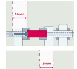
Can bottom forming on one working station with a bottom forming punch
