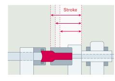
Different lengths of the stroke can be chosen for shaping the can body
