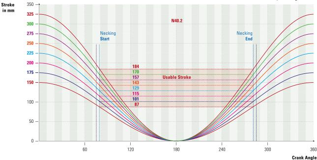
Different characteristic lines can be chosen to obtain the necessary working stroke.
