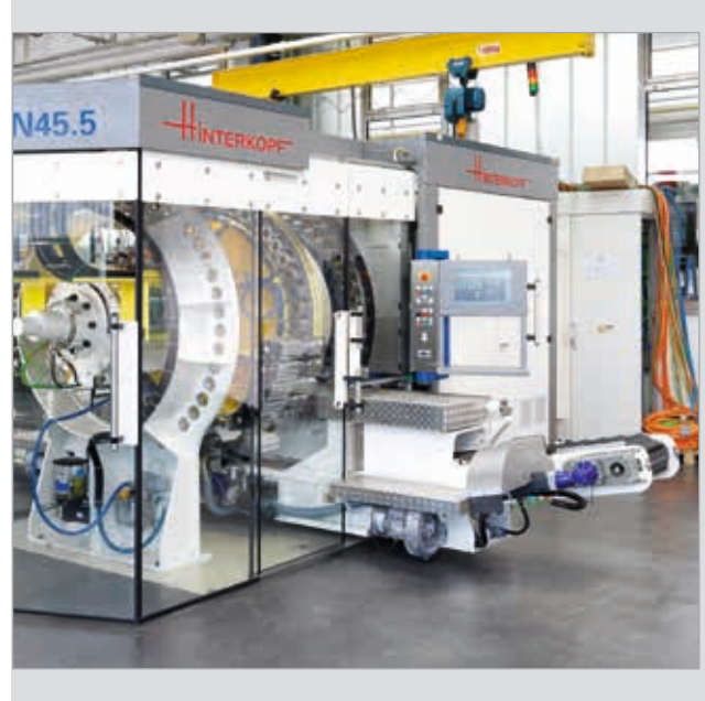
Moveable and adjustable (in height and angle) infeed and exit conveyors for good access.
